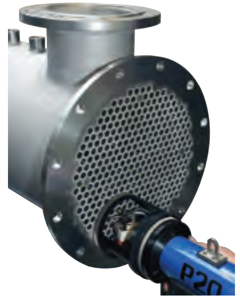
Automated tube end welding and 100% inspection
